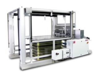
The aluminum is cut into 50-in. sheets. A set of grippers holds the material coming from the cut-to-length unit. Once the material is held in the gripper, the cut-to-length unit indexes the material; at the same time, the linear actuators move the material into position, over the stack.
